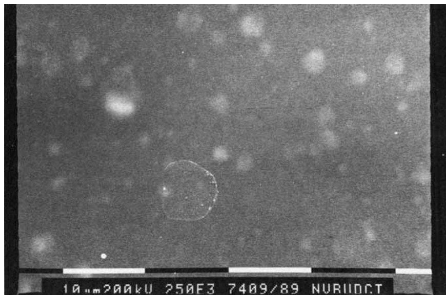
Figure 3 SEM micrograph of \text{FeCl}_3 -doped PAN exposed for 15 min.
